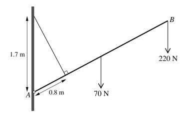
A uniform beam AB has length 2 m and weight 70 N. The beam is hinged at A to a fixed point on a vertical wall, and is held in equilibrium by a light inextensible rope. One end of the rope is attached to the wall at a point 1.7 m vertically above the hinge. The other end of the rope is attached to the beam at a point 0.8 m from A. The rope is at right angles to AB. The beam carries a load of weight 220 N at B (see diagram).
